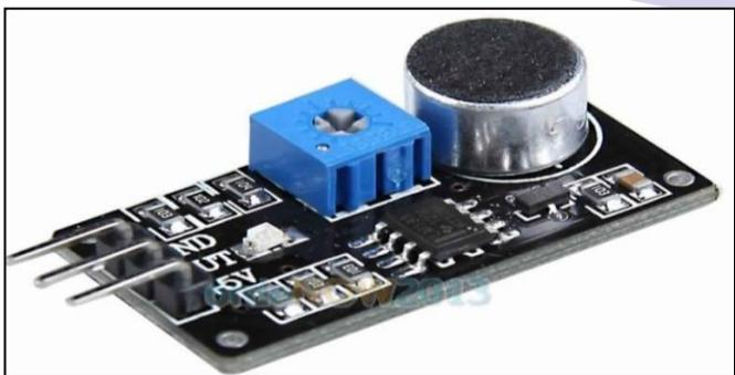
Fig 5: clap detecting sensor
